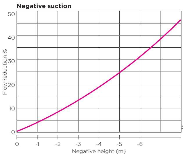
Lifting the liquid from a negative height reduces the flow of the pump as in standard circumstances (flooded suction).
