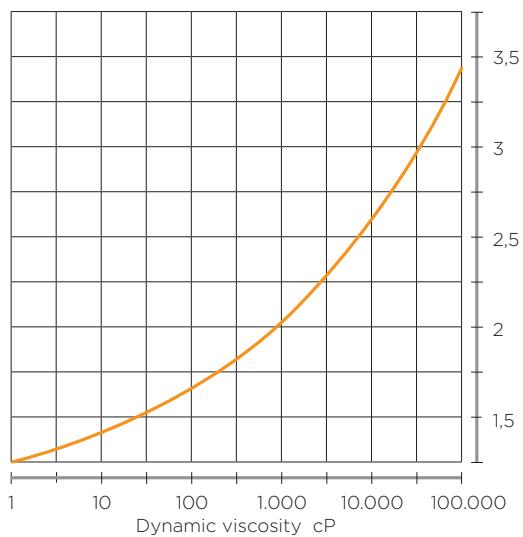
Multiply coefficient for pipeline diameter referred to a non viscous fluid and constant hydraulic losses.
